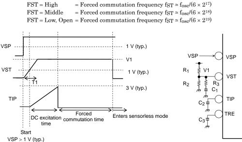
3) Timing Diagram of the Startup Operation (CW\_CCW = Low: Clockwise rotation)
