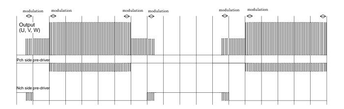
Timing diagrams of commutation waveforms (CW\_CCW = Low: Clockwise rotation)
