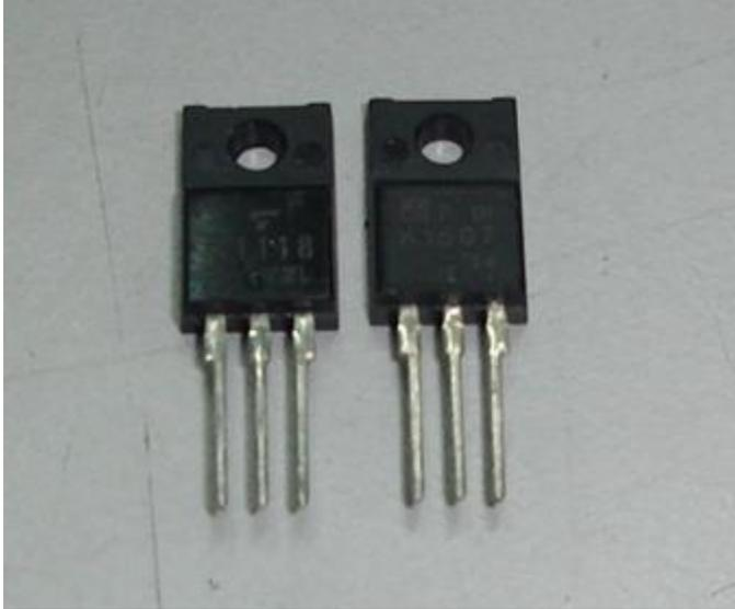
The right way of testing mosfet transistor is to use an analog multimeter. Mosfet stand for Metal oxide semiconductor field effect transistor or we just called it fet. Switch mode power supply and many other circuits uses fet transistors as part of a circuit. Mosfet failure and leakage are quite high in a circuit and you need to know how to accurately test it.
